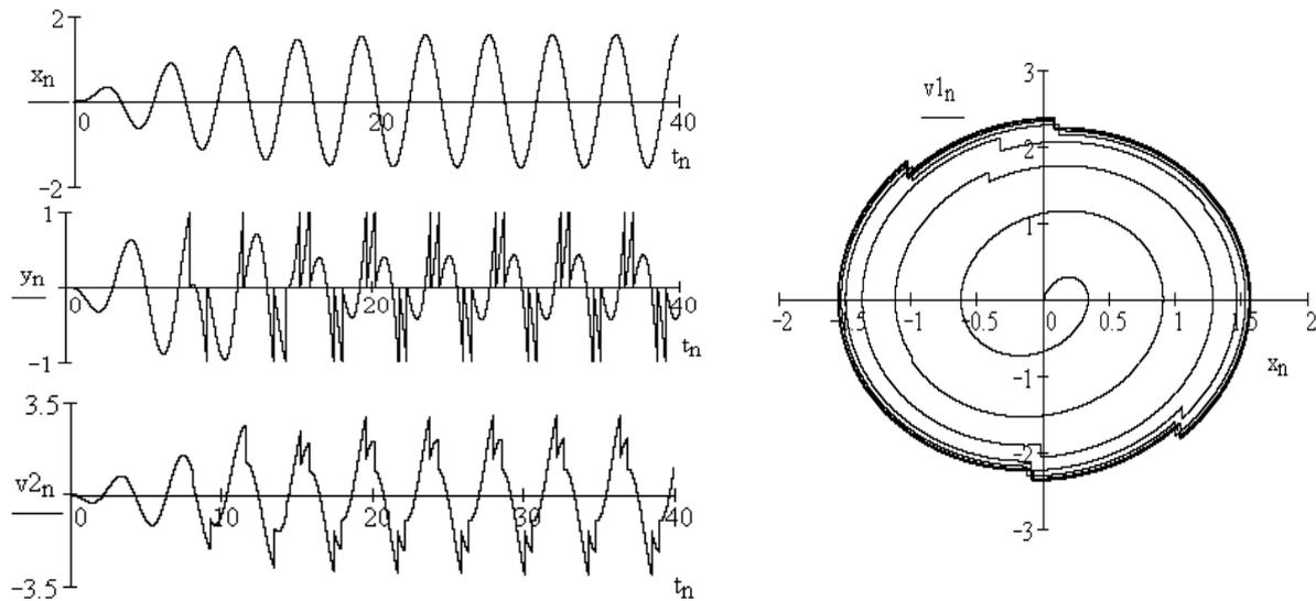
Fig. 12. Plots of dependence of motion parameters on time:  $x=x(t)$ ,  $y=y(t)$ ,  $v_2r=v_2r(t)$  and phase map for classical impact absorber in case of:  $\Omega=1.5$ ,  $\lambda=1.5$ ,  $c=1$ ,  $\mu=0.04$ ,  $r=0.6$ .
