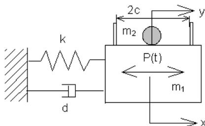
Fig.11. Model of classical impact absorber.
