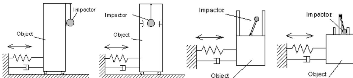
Fig.3. Pendulum impact absorber
