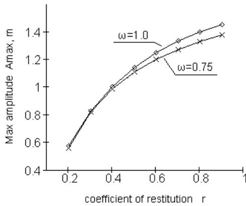
Fig.9. Maximal amplitude  $A_{max}$  in relation to coefficient of restitution  $r$  for single impact pendulum absorber ( $\mu=0.04$ ,  $r=0.6$ ).
