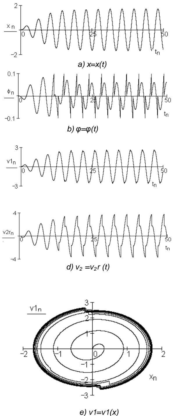
Fig. 6. Plots of dependence of the motion parameters on time and phase map for double-impact absorber in case of:  $\Omega=1.5$ ,  $\lambda=1.5$ ,  $\omega=0.75$ ,  $\alpha=0.1$ ,  $\mu=0.04$ ,  $r=0.6$ .
