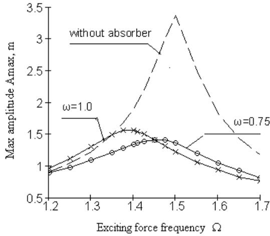
Fig.7. Maximal amplitude  $A_{max}$  in relation to exciting force frequencies  $\Omega$  for single impact pendulum absorber ( $\mu=0.04$ ,  $r=0.6$ ).
