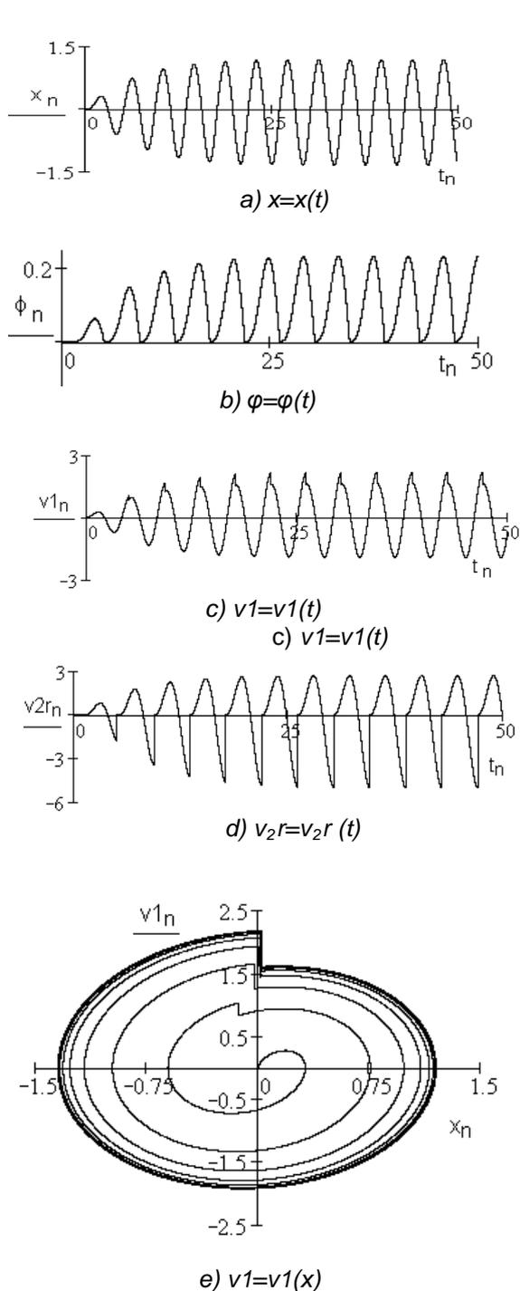
Fig. 5. Plots of dependence of the motion parameters on time and phase map for single-impact absorber in case of:  $\Omega=1.5$ ,  $\lambda=1.5$ ,  $\omega=0.75$ ,  $\mu=0.04$ ,  $r=0.6$ .
