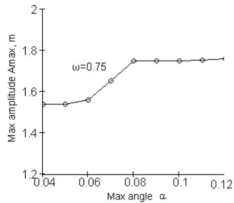
Fig.10. Maximal amplitude  $A_{max}$  depending on pendulum clearance angle  $\alpha$  ( $\mu=0.04$ ,  $r=0.6$ ) for multi-impact absorber shown in Fig.4b.
