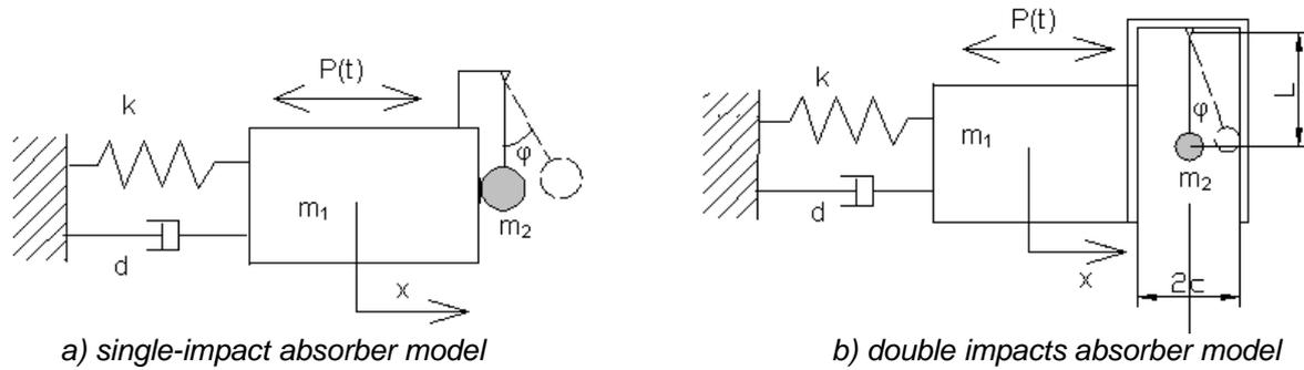
Fig.4. Model of the pendulum impact absorber.
